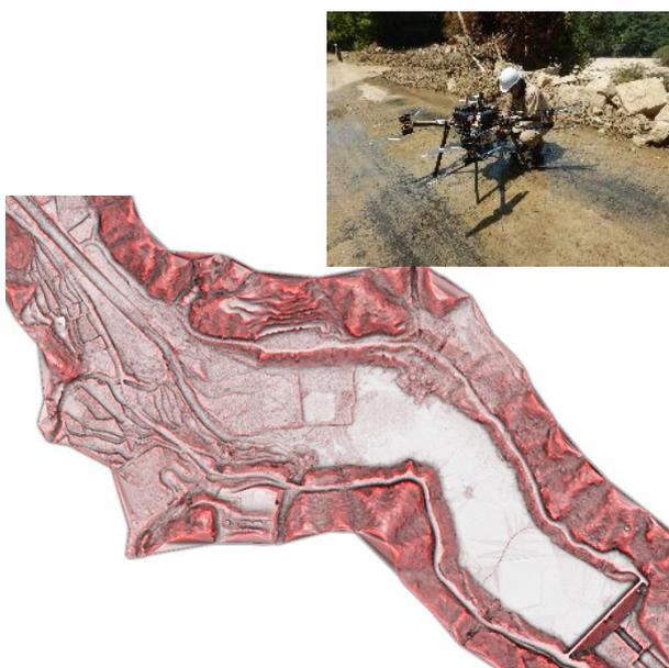
図-5.2.2 UAV レーザ測量成果
