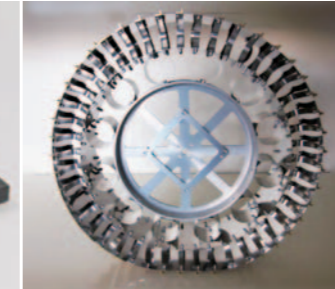
図9 金属製弾性車輪 © JAXA
