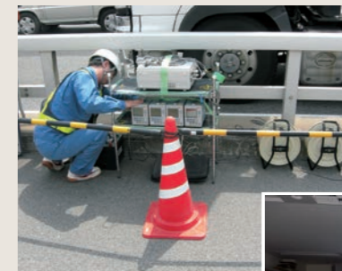
橋梁の振動計測
